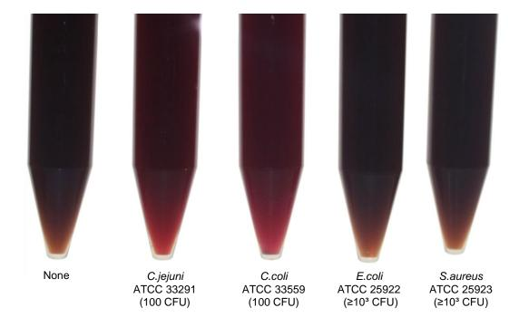
Incubation conditions :  $42 \pm 2^{\circ}$ C / 48 - 72 hours under microaerobic condition
